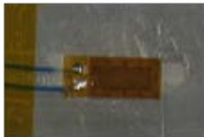
Figure 3: Strain gauge.
