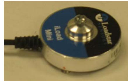
Figure 2: Load cell.
