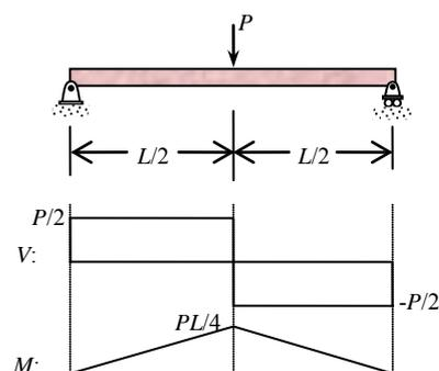
The first step of the analysis is to find the maximum deflection of the beam. The equation for the elastic curve is found through the double integration approach. From a free body diagram of the beam to the left of the point load, i.e.  $0 \leq x \leq L/2$ , the following expressions can be written:
