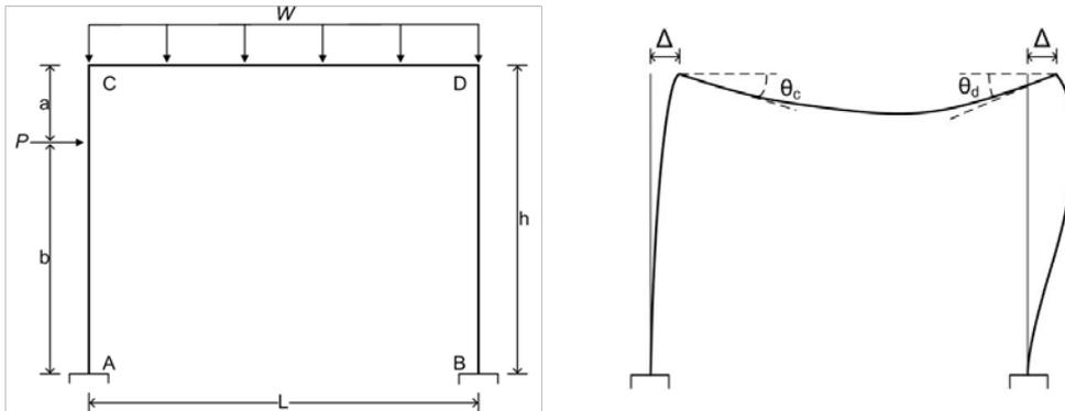
Figure 10: Portal frame with a before and after view of its configuration due to shown loading.
