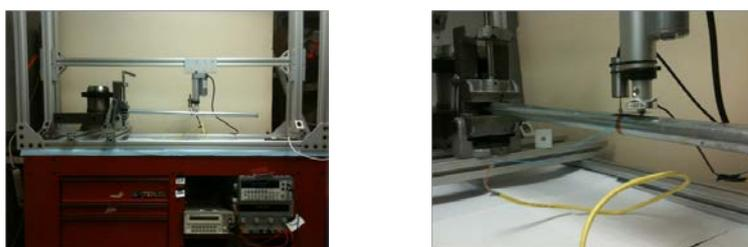
Figure 5: SEE test on a tubular cantilevered beam with point load at midspan.
